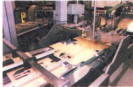
High speed, complex motion and logic are managed by a single controller for this two-piece cardboard converter of open-basket carriers from Roberts PolyPro. Source: Rockwell Automation.
